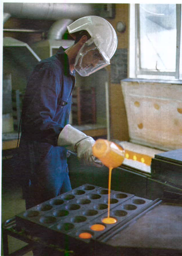
Fire Assayer pours liquid rock and molten lead containing gold into iron mould.
