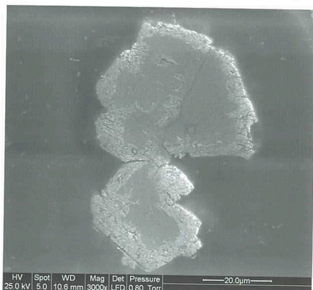
Fig. 6. Environmental SEM image of the cross-section of a relatively small industrial alumina grain showing significant phase differentiation across the section; phase distribution is influenced by the calcination conditions and calciner technology.
